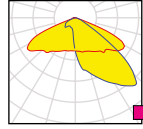
MEW Extremely low glare fulfilling EN13201 M-class requirements for wet road surfaces in North Europe
