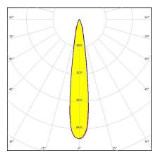
Dimensions: 74.9 mm x 74.9 mm Height: 9.50 mm ~15° spot beam
