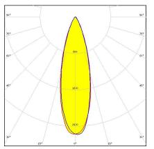
Dimensions: 74.9 mm x 74.9 mm Height: 9.50 mm ~30° medium beam
