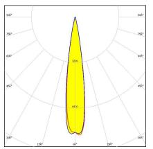
Dimensions: 21.7 mm x 21.7 mm Height: 6.60 mm ~15° spot beam
