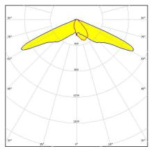
Dimensions: 13.9 mm x 13.9 mm Height: 5.32 mm Asymmetric IESNA Type I (short) beam
