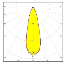
Dimensions: 90.0 mm x 90.0 mm Height: 39.15 mm ~25° spot beam. Compatible with up
