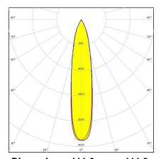
Dimensions: 111.0 mm x 111.0 mm Height: 80.00 mm ~18° smooth spot beam
