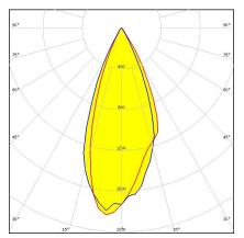
Dimensions: 21.6 mm x 21.6 mm Height: 14.70 mm ~40° wide beam optimized for CREE XP-E. 14.7 mm high assembly with installation tape.
