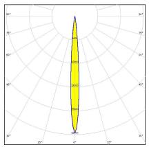
Dimensions: 21.6 mm x 21.6 mm Height: 15.10 mm ~9.6° spot beam optimized for LedEngin LZ1(00XW00). 15.1 mm high assembly.
