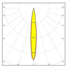
Dimensions: 21.6 mm x 21.6 mm Height: 14.80 mm ~14° diffused spot beam optimized for LUXEON Rebel ES. 14.8 mm high assembly with installation tape.
