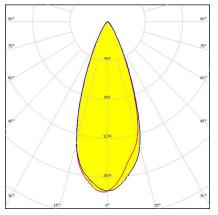
**Dimensions: 21.8 mm x 21.8 mm Height: 14.70 mm** ~40° wide beam with light, black holder. Assembly with location pins and installation tape.
