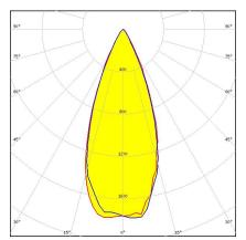
Dimensions: 21.6 mm x 21.6 mm Height: 14.70 mm ~40° wide beam optimized for CREE XP-E. 14.7 mm high assembly.
