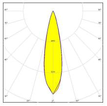
Dimensions: 21.6 mm x 21.6 mm Height: 14.04 mm ~14° diffused spot beam optimized for CREE MC-E. 14.04 mm high assembly
