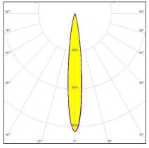
Dimensions: 21.6 mm x 21.6 mm Height: 14.70 mm ~14° diffused spot beam optimized for CREE XP-E. 14.7 mm high assembly
