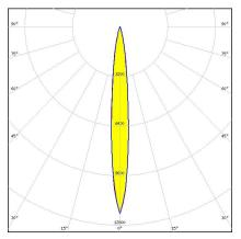
Dimensions: 21.6 mm x 21.6 mm Height: 14.60 mm ~9.6° spot beam optimized for Osram Golden Dragon+. 14.6 mm high assembly with installation tape.
