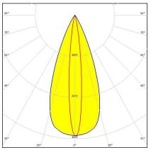
Dimensions: 21.6 mm x 21.6 mm Height: 14.70 mm ~10° x 40° oval beam optimized for CREE XP-E. 14.7 mm high assembly
