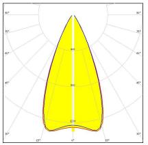
Dimensions: 21.6 mm x 21.6 mm Height: 14.30 mm ~40° wide beam optimized for LUXEON Rebel. 14.3 mm high assembly.
