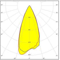
Dimensions: 21.6 mm x 21.6 mm Height: 14.30 mm ~40° wide beam optimized for Osram
