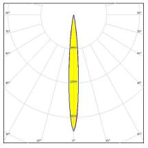
Dimensions: 21.6 mm x 21.6 mm Height: 14.30 mm ~9.6° spot beam optimized for Osram Oslon Square EC. 14.3 mm high assembly.
