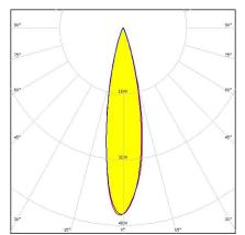
Dimensions: 21.8 mm x 21.8 mm Height: 14.70 mm ~20° medium beam with light, black holder. Assembly with location pins and installation tape.
