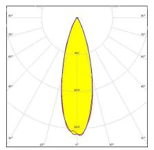
Dimensions: 21.6 mm x 21.6 mm Height: 14.04 mm ~40° wide beam optimized for CREE MC-E. 14.04 mm high assembly with installation tape.
