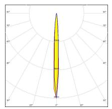
Dimensions: 21.6 mm x 21.6 mm Height: 14.30 mm ~8.5° spot beam optimized for Osram Oslon Square EC. 14.3 mm high assembly.
