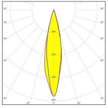
Dimensions: 21.6 mm x 21.6 mm Height: 14.40 mm ~25° medium beam optimized for
