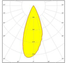
Dimensions: 21.6 mm x 21.6 mm Height: 14.60 mm ~40° wide beam optimized for CREE XB-D. 14.6 mm high assembly with
