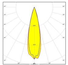
Dimensions: 21.8 mm x 21.8 mm Height: 14.70 mm ~20° medium beam with light, black holder. Assembly with installation tape.
