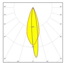
Dimensions: 21.6 mm x 21.6 mm Height: 14.60 mm Asymmetric beam for wall-washing and
