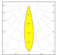
Dimensions: 21.6 mm x 21.6 mm Height: 14.70 mm ~25° medium beam optimized for CREE
