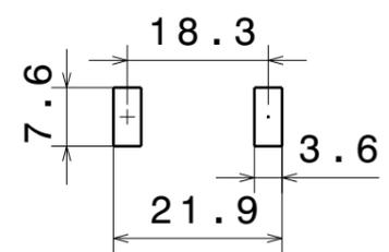
Clip reference distance after soldering
