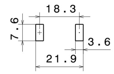
Clip reference distance after soldering
