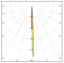
Dimensions: 50.0 mm x 50.0 mm Height: 53.00 mm ~3° spot beam
