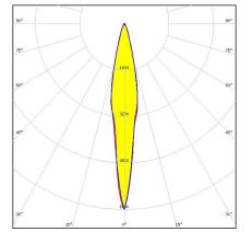
Dimensions: 280.0 mm x 35.0 mm Height: 14.51 mm ~20° beam. 8X1 variant.
