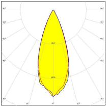
Dimensions: 280.0 mm x 35.0 mm Height: 15.00 mm ~40° beam. 8X1 variant.
