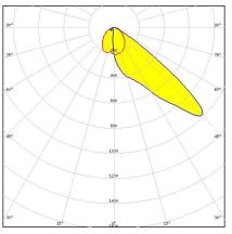
**Dimensions: 280.0 mm x 35.0 mm Height: 20.65 mm** Forward throwing beam with peak in 45°.
