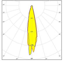
Dimensions: 72.8 mm x 72.8 mm Height: 11.00 mm ~20° medium beam
