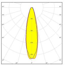
Dimensions: 72.8 mm x 72.8 mm Height: 11.10 mm ~25° medium beam
