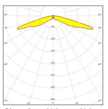
Dimensions: 21.6 mm x 21.6 mm Height: 7.30 mm Asymmetric beam. Assembly with installation tape.
