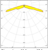
Dimensions: 33.0 mm x 25.0 mm Height: 11.00 mm Asymmetric beam. Assembly with installation tape.
