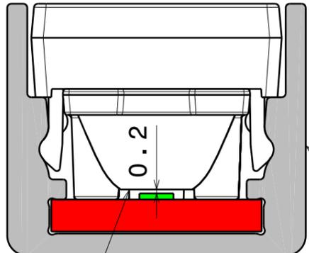
Ensure there's gap between LED and lens for fluent assembly result.
