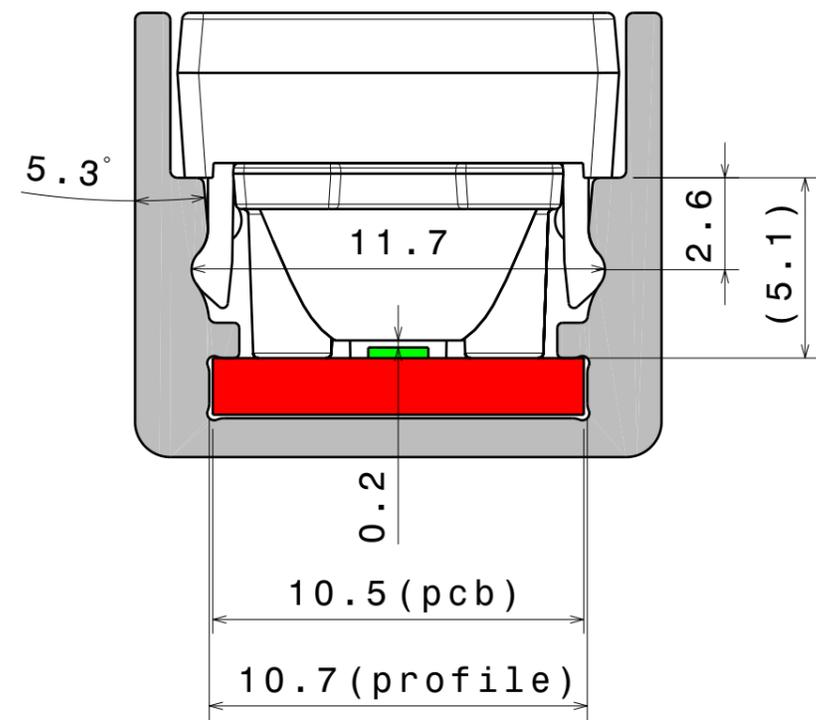
Adjust dimension (5.1) based on used LED type.
