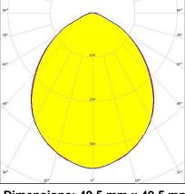
Dimensions: 49.5 mm x 49.5 mm Height: 7.12 mm ~90° wide beam for industrial applications
