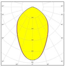
Dimensions: 49.5 mm x 49.5 mm Height: 7.12 mm ~60° medium beam for industrial applications
