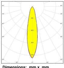
Dimensions: mm x mm Height: mm ~24° medium beam
