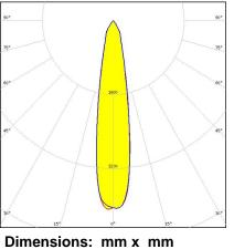
Dimensions: mm x m Height: mm ~15° spot beam
